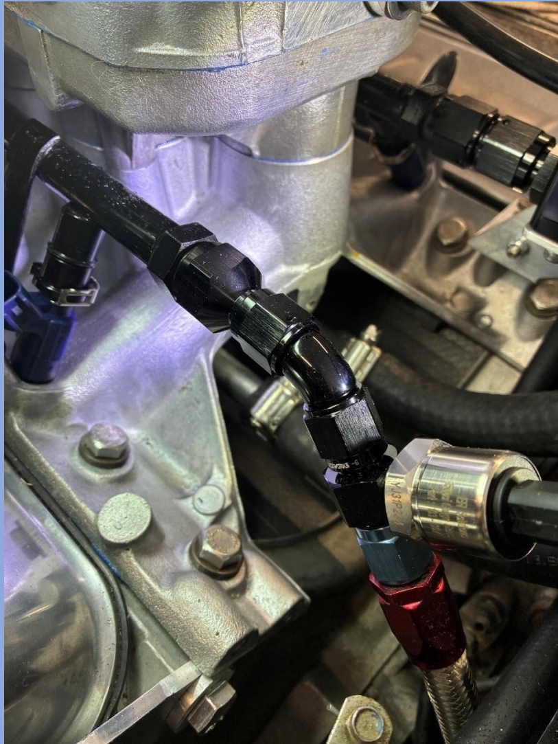
Modified Fuel Rail with Flare fittings & fuel Pressure Sensor
